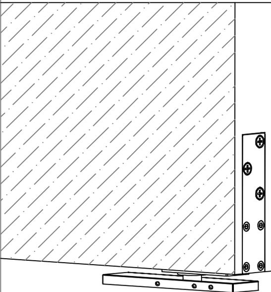
5. Ensure the alignment of door panel by adjusting the set screws on the base seat.
