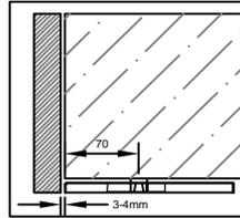
1. Determine the position of floor hinge to be installed and ensure the horizontal position of base seat. Install the cover plate after base seat is fixed .
