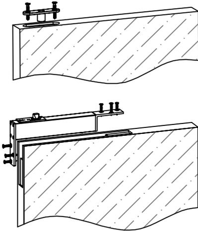
3. Fix the floor hinge and top pivot onto door leaf by wood screws.
