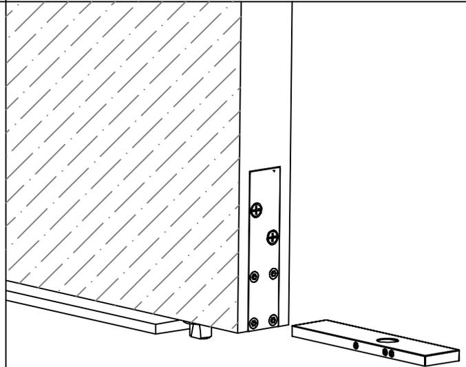
4. Install the floor hinge onto base seat and fix the top pivot with ceiling pivot. At this step, the setting screws on base seat should be loosen.
