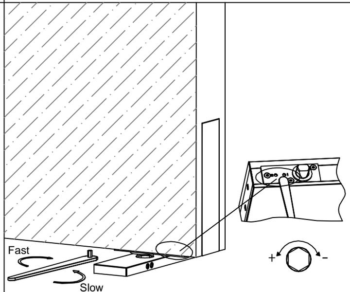
6. Adjust the required closing speed by allen key, and installation is done.
